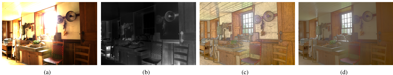
Figure 1: (a) the input high dynamic range (HDR) image. (b) the guided image constructed by our approach. Mathematically, the guided image can be regarded as a scalar matrix which map the HDR luminance channel \mathbf{I}^h into low dynamic range (LDR) luminance channel \mathbf{I}^l simply by \mathbf{I}^l = \mathbf{P} \cdot \mathbf{I}^h . The scalar matrix \mathbf{P} is calculated per pixel with local mean and variance in the luminance channel of the input HDR image. Bright regions in the guided image indicate that the same areas of the input HDR image should be enhanced, otherwise should be compressed. (c) our enhanced result in details ( \lambda_1 = 0.6, \lambda_2 = 0.3 ). (d) our natural result ( \lambda_1 = 0.6, \lambda_2 = 0.1 ).
